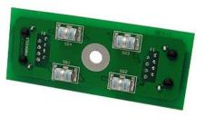
HGLN-CAT6JT utilizes gas discharge tubes on each pair for superior power handling capability. This protector is compatible with 802.3af/at Power-over-Ethernet (PoE) devices. It supports both PoE mode A and B for power.
